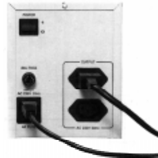
fig. J2-19: ready-to-use UPS unit.
